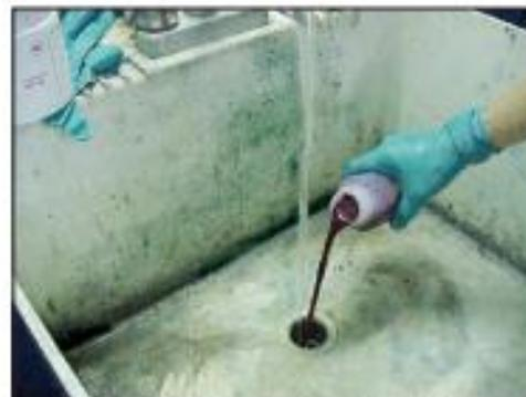
Figure 63: Dye Testing Plumbing (NEIWPCC, 2003)
